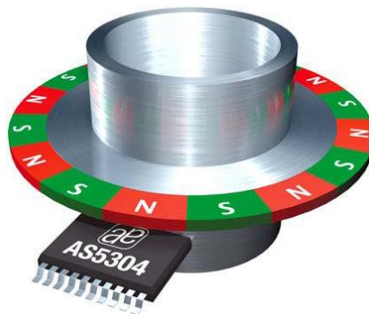
Figure 12: A common off-axis encoder (AS5304, 12-bit of resolution)
