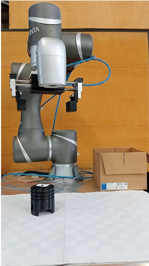
(a) Robot rotates gripper according to previously evaluated object orientation.
