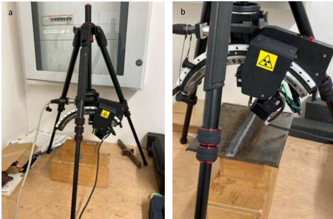
Figure 18 Representation of portable XRD diffractometer (a) XRD diffractometer sampling on MIG welded plates (b)
