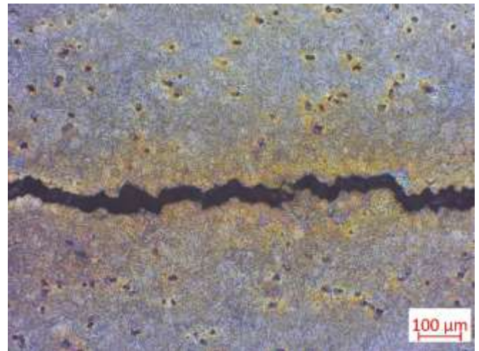
Figure 75 Cracks generated on the welded sample after quenching heat treatment
