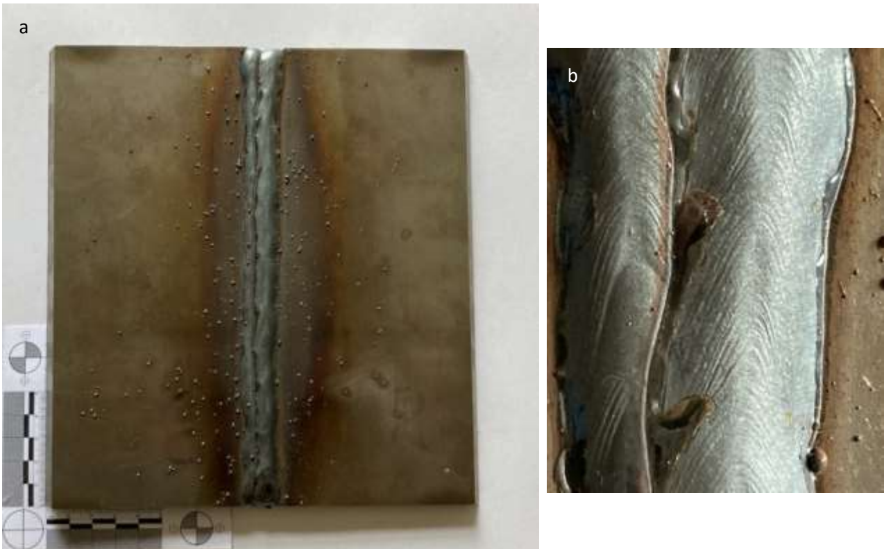
Figure 27 Weld bead obtained with MIG process (a), glassy product on the weld bead (b)
