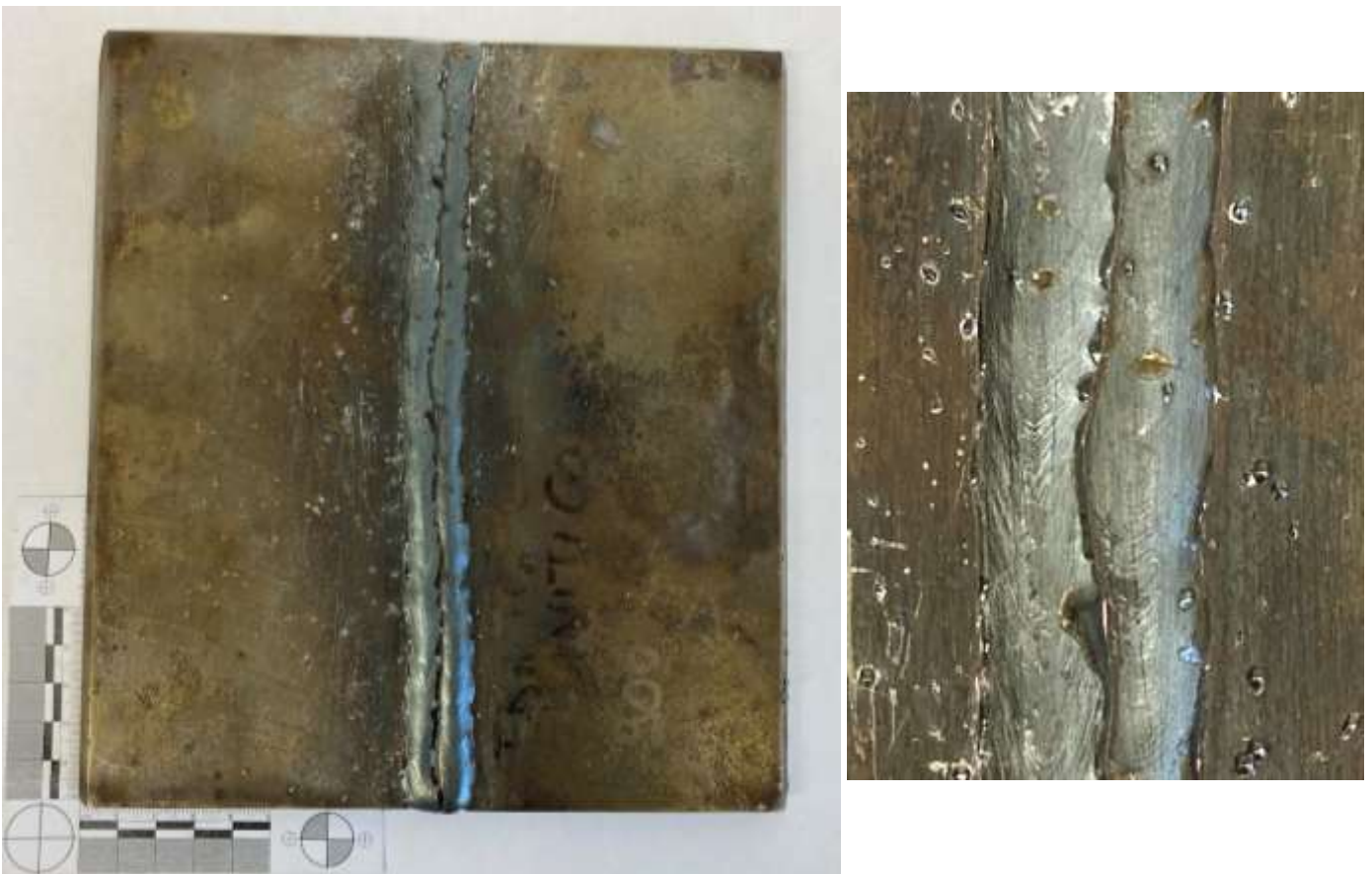
Figure 104 Pictures of austempered steel plates welded with MIG welding process
