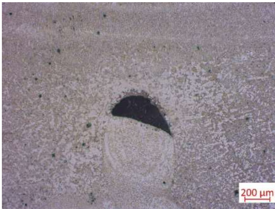
Figure 73 Pore defect detected in the fusion zone of annealed sample
