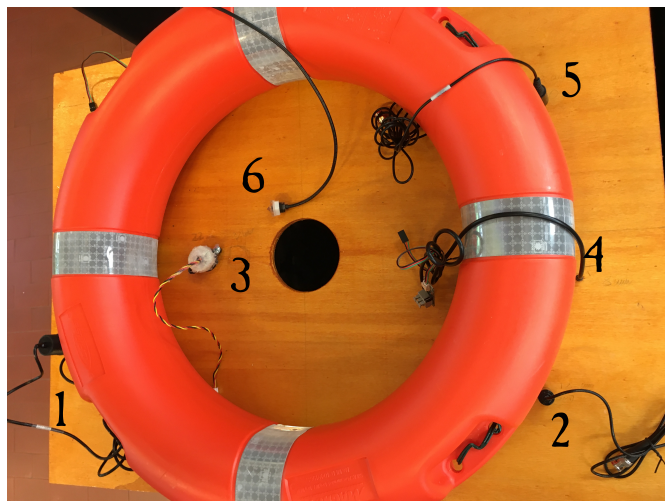
Figure 6.5: Bottom panel of SENSWICH (top wooden panel removed) with sensors: 1. pH sensor, 2. EC sensor, 3. Turbidity sensor, 4. Temperature sensor, 5. DO sensor, 6. liquid Level Sensor.
