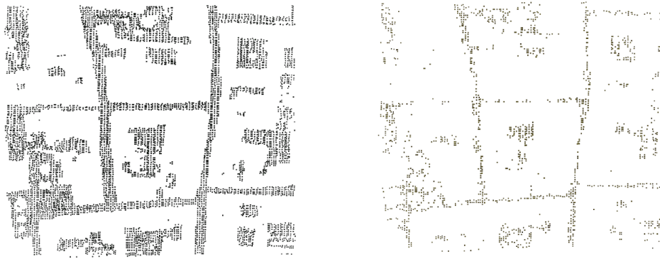
Figure 4.6: Left image: before erosion, Right image: after erosion
