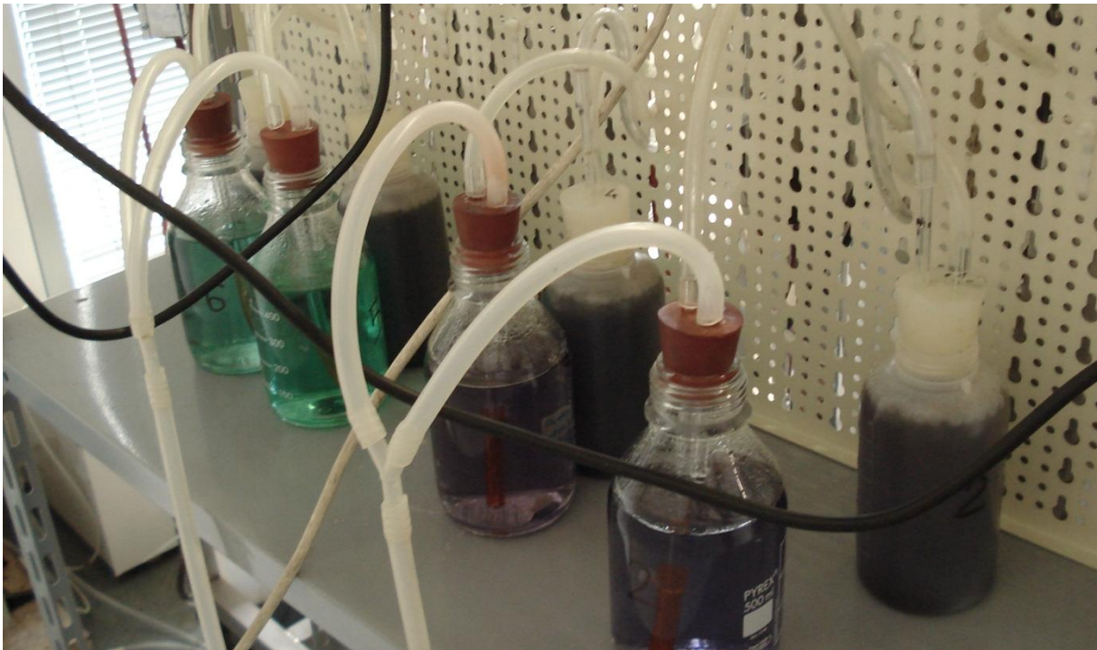
Figure 3 – Scrubbers filled with boric acid for the outflowing gas washing in order to quantify the content of ammonia-nitrogen
