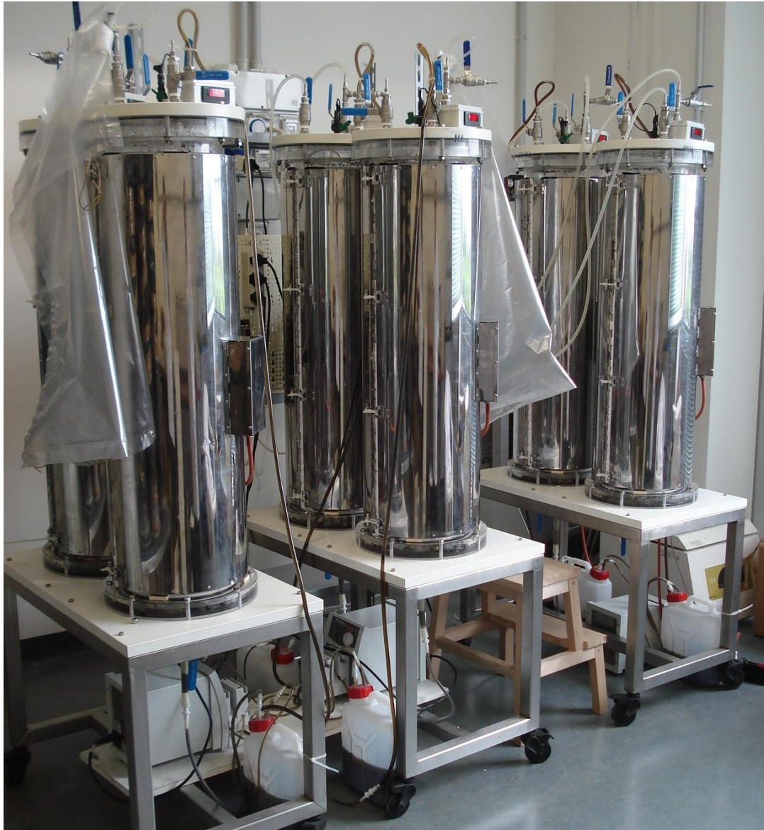
Figure 1 – Reactors with thermal insulated armor, provided with bags for the biogas collection
