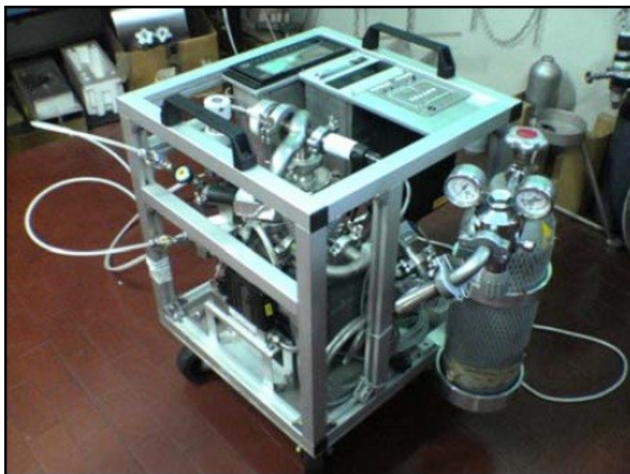
Figure 4.2 – Vacuum and gas flow system used to perform microdosimetric measurements
