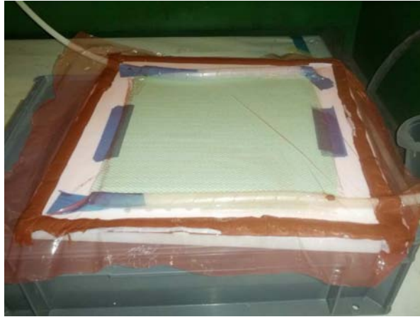
Fig. 3.1: VARTM laminating process lay-up
