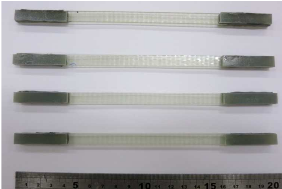
Fig. 3.12: Specimens of dimension 200 mm x 8mm end-tabbed
