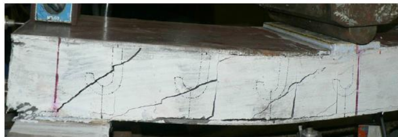
(b) Shear cracks extend and widen at 63 kN load and 31 mm deflection.
