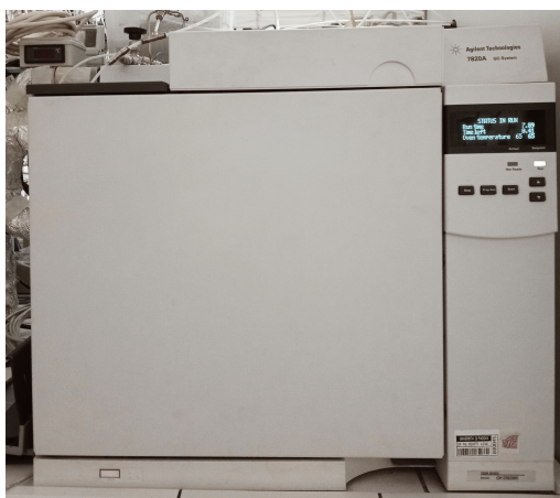
Figure 2.12: Gas chromatograph used to analyse the gaseous mixture.
