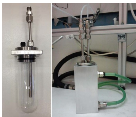
Figure 2.14: Condenser (right) and its internal structure (left) [35].
