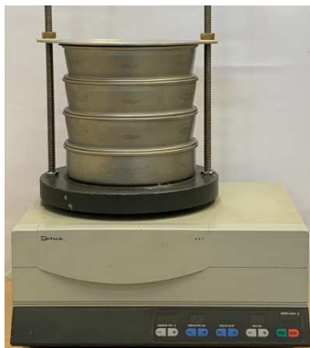
Figure 2.4: Vibratory sieve shaker used for sieving the grind SiC and Catalyst.
