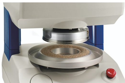
Figure 2.5. Brookfield powder flow tester (PFT) with powder sample in an annular shell cell going to be compressed by a compression lid vertically downward into it ( https://store.brookfieldengineering.com/pft-powder-flow-tester ).
