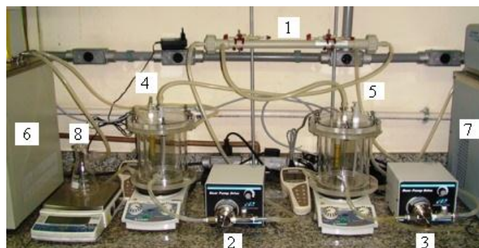
Figure 4.3 Bench-scale unit: 1) Membrane module, 2) draw pump, 3) sucrose solution pump, 4) Draw tank, 5) Sucrose solution tank, 6) Criostatic bath for draw, 7) Crisostatic bath for sucrose solution, 8) Balance with permeated liquid.
