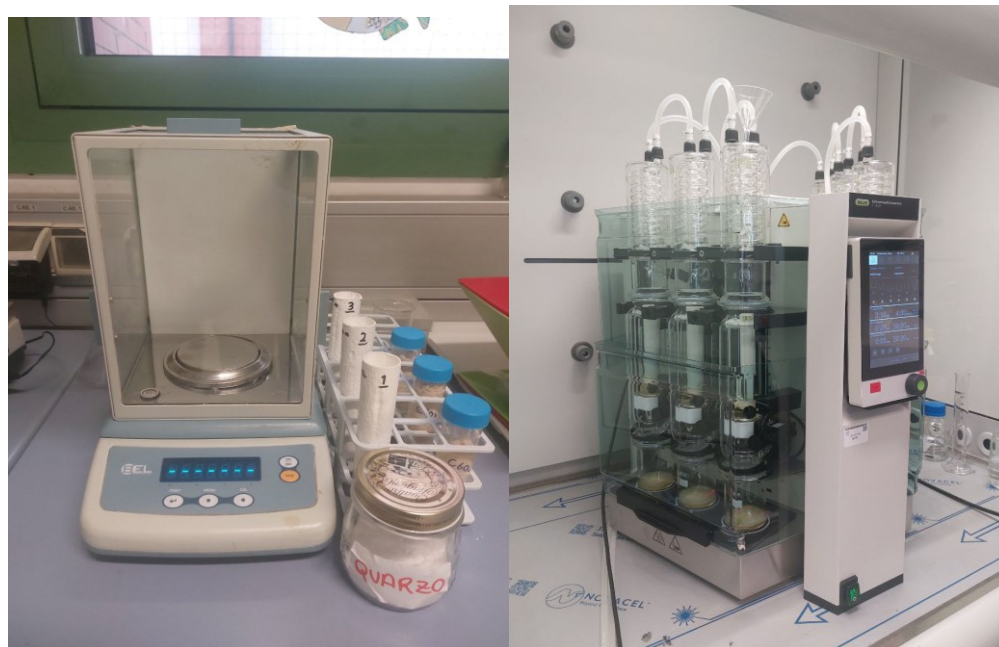
Figure 4.18. Fat extraction setup: Sample preparation station including extraction thimbles, and quartz sand (Left); The Buchi Universal Extractor E-800 unit during the extraction process (Right)
