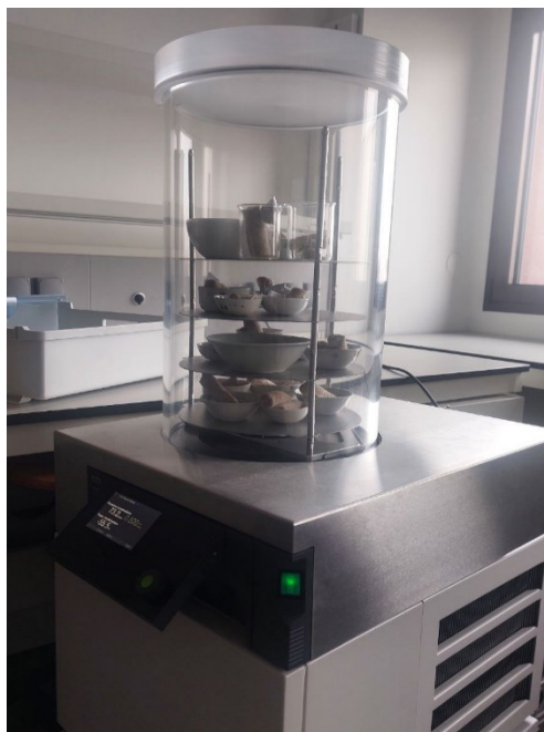
Figure 4.15. Lyophilization of fish samples using a laboratory freeze dryer (Lyovapor™ L-200, BUCHI)
