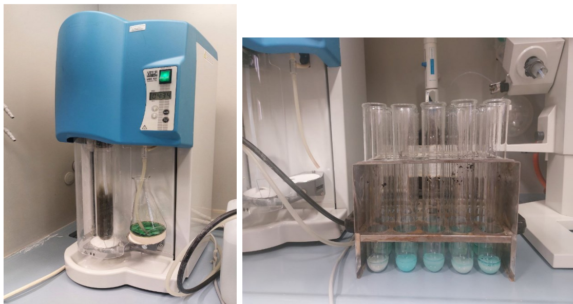
Figure 4.17. The ammonia distillation process using the VELP UDK 127 unit (Left), and Digested samples showing the characteristic clear blue-green color (Right)
