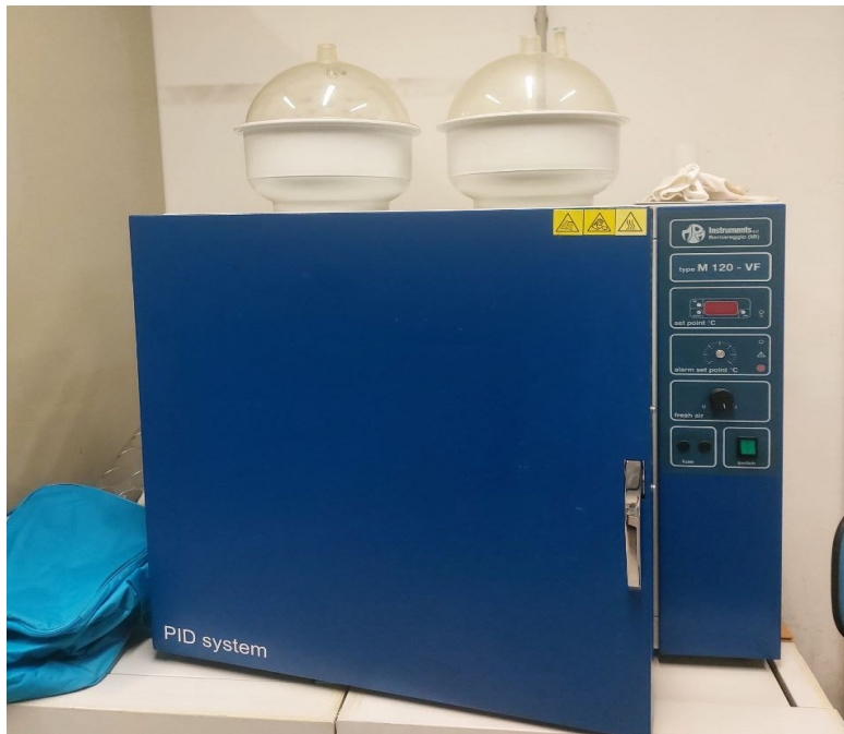
Figure 4.11. Experimental equipment for moisture content determination: drying oven and glass desiccators
