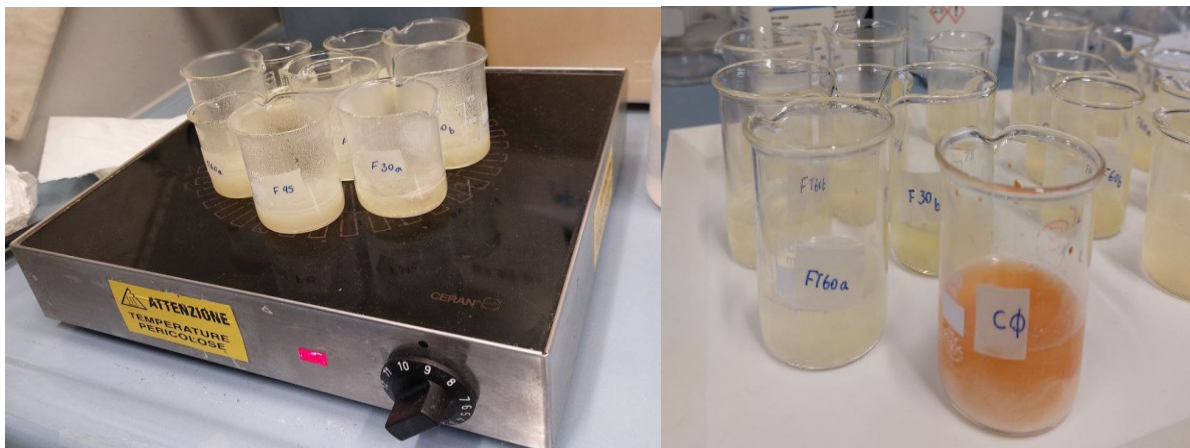
Figure 4.21. Determination of chlorides: Sample boiling step on the hot plate (Left); the endpoint of the titration (Right)
