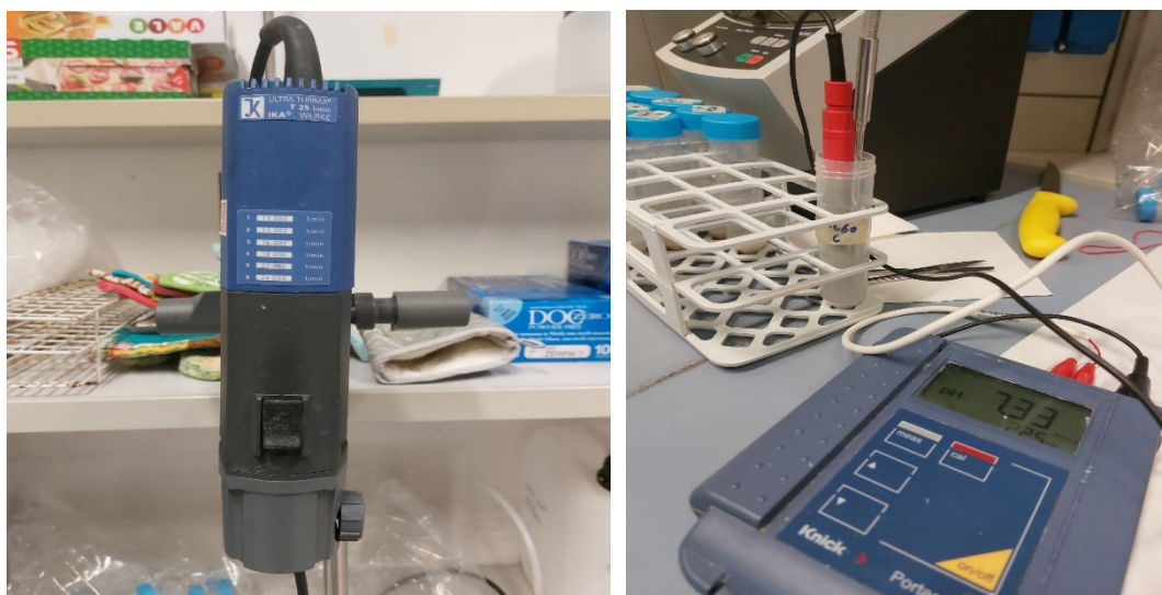
Figure 4.9. Experimental setup for sample preparation, including the ULTRA-TURRAX T25 basic homogenizer (Left) and the KNICK Portamess pH meter (Right)
