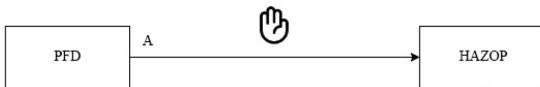
Figure 14: Starting from the available documentation (e.g., a process flow diagram), a traditional HAZOP analysis (preHAZOP in this case) is performed (Scenario 1).
