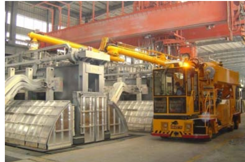
(b) Potcel feeding operation
