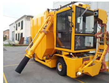
(f) Taphole breaking and covering
