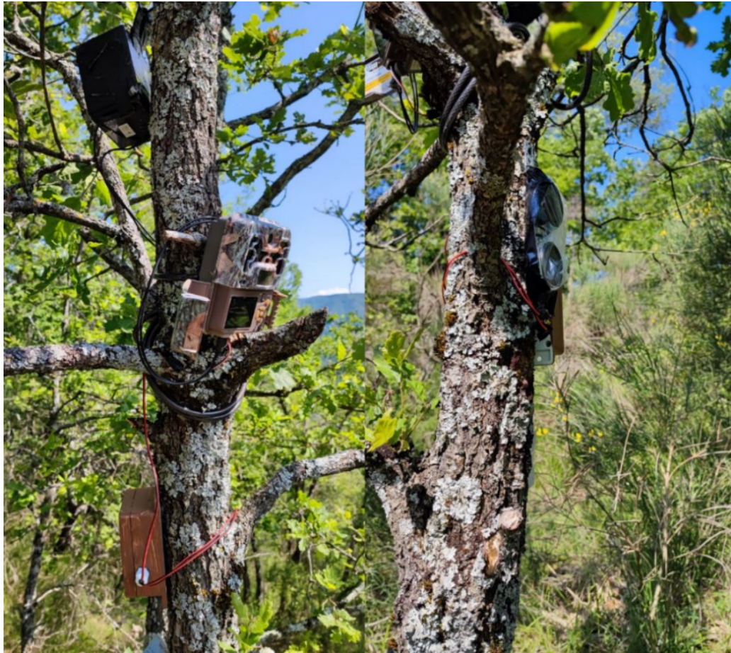
Figure 2. Camera traps (Browning Spec Ops Advantage BTC-8A, left) with external speakers (right) used to play human voice and bird sounds during the test.
