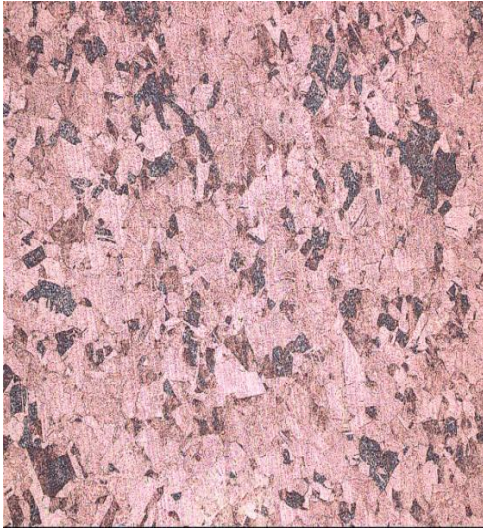
Fig. 41: LOM image, heat affected zone 100X Weld 1
