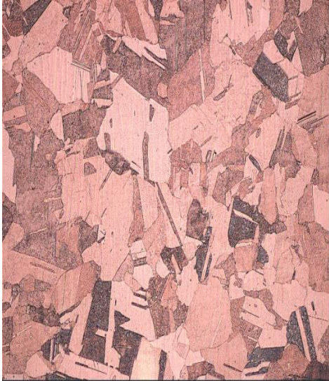
Fig.40: LOM image, base material 100X Weld 1
