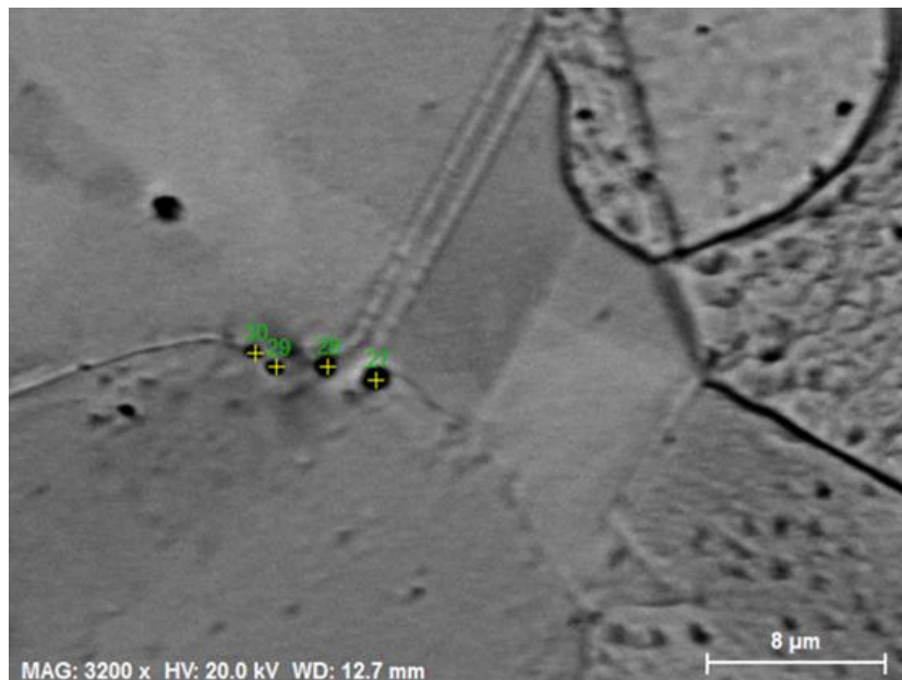
Fig. 54: Inclusions after electrolytic polishing and etching
