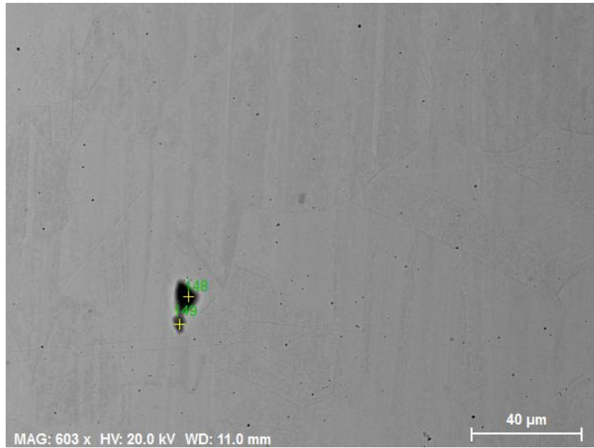
Fig. 50: Inclusions after oxides polishing and chemical etching.
