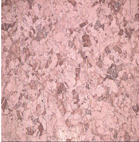
Fig. 42: LOM image, friction zone 100X Weld 1
