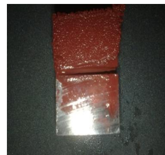
Fig. 33: Stainless steel cathode covered in copper
