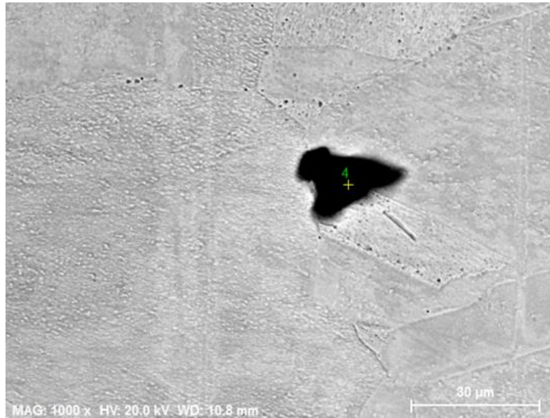
Fig. 49: Dirt inclusion after mechanical polishing and chemical etching.
