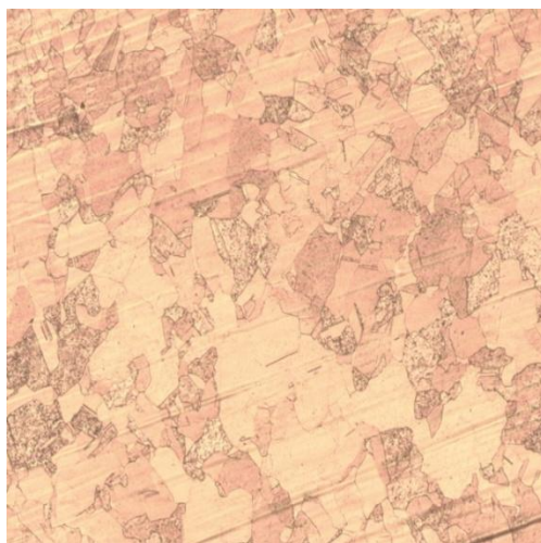
Fig. 44: LOM image, heat affected zone, 100X Weld 2
