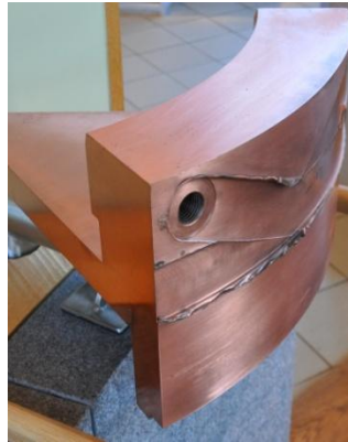
Fig. 23: Segment of lid and but welded together
