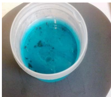
Fig.34: Electrolytic bath with copper residuals
