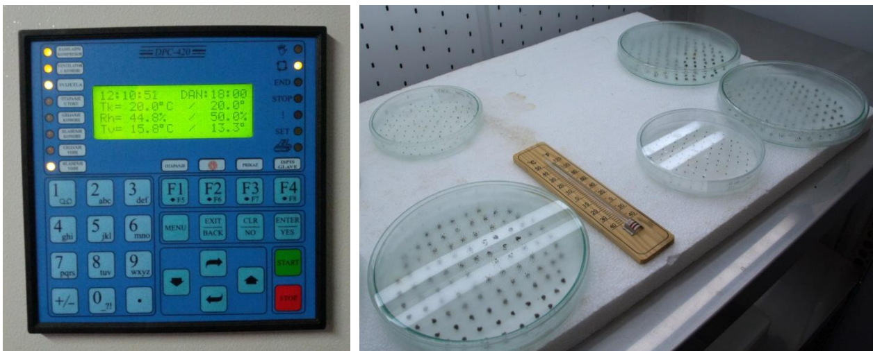
Figure 15. Germinator's settings for 20°C and Petri dishes inside the germinator ( photos: Dario Magosso ).
