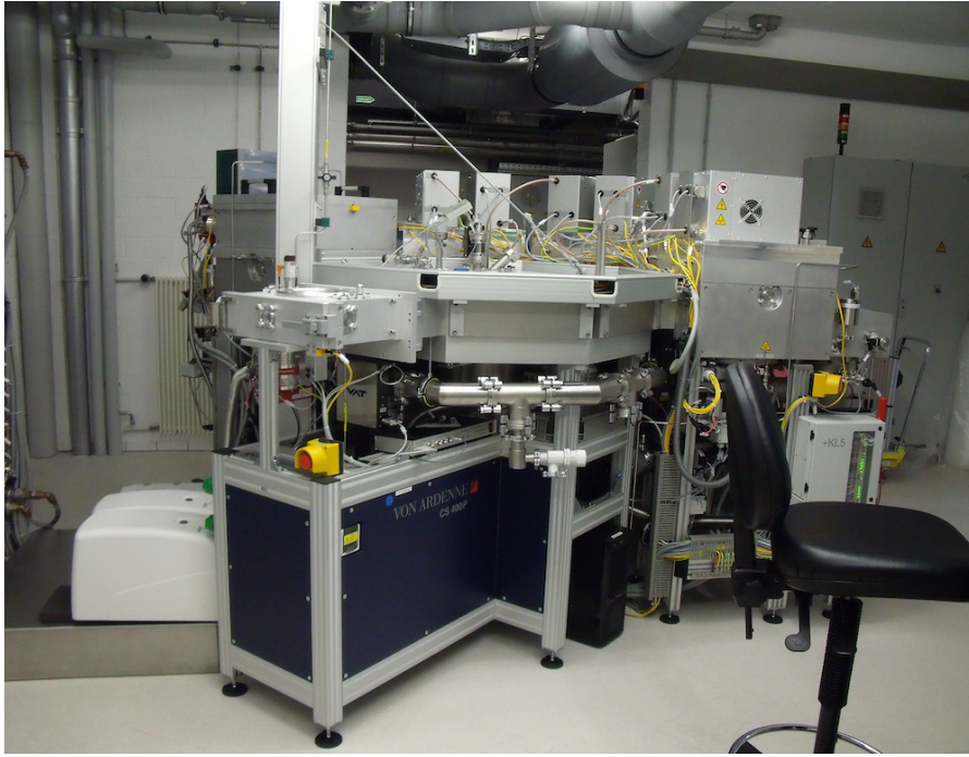
Figure 4.10: The PECVD system. - The PECVD system used in this work, from Von Ardenne.
