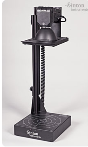
Figure 3.1: Sinton Instrument WCT-120 - Picture of the tool used for lifetime and implied V_{OC} measurement.
