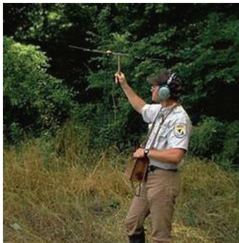
Picture 5.1 - Traditional VHF telemetry uses a directional, hand-held antenna to receive transmissions.
