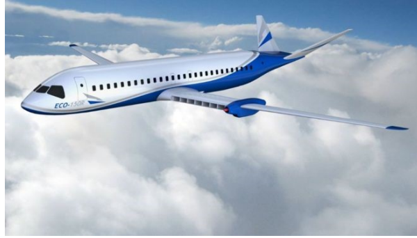
Figure 0.2: Example of distributed propulsion ESAero eco-150
