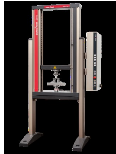
Figure 45. ZwickRoell 10 kN RetroLine [97].
