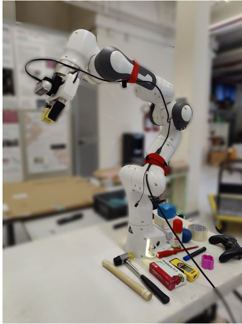
Figure 4.1: 7-DoF Franka-Emika Panda robot used for the experiments.
