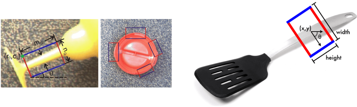
Figure 2.7: Both images show the 5-DoF rectangles used to represent a grasp in the image plane. On the left, the one considered by [30]. On the right the one by [47].
