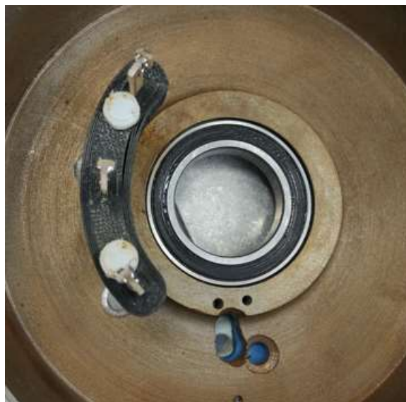
Figure 4.5 - View on the Hall-effect sensors placed on the end shield of the IPM machine.
