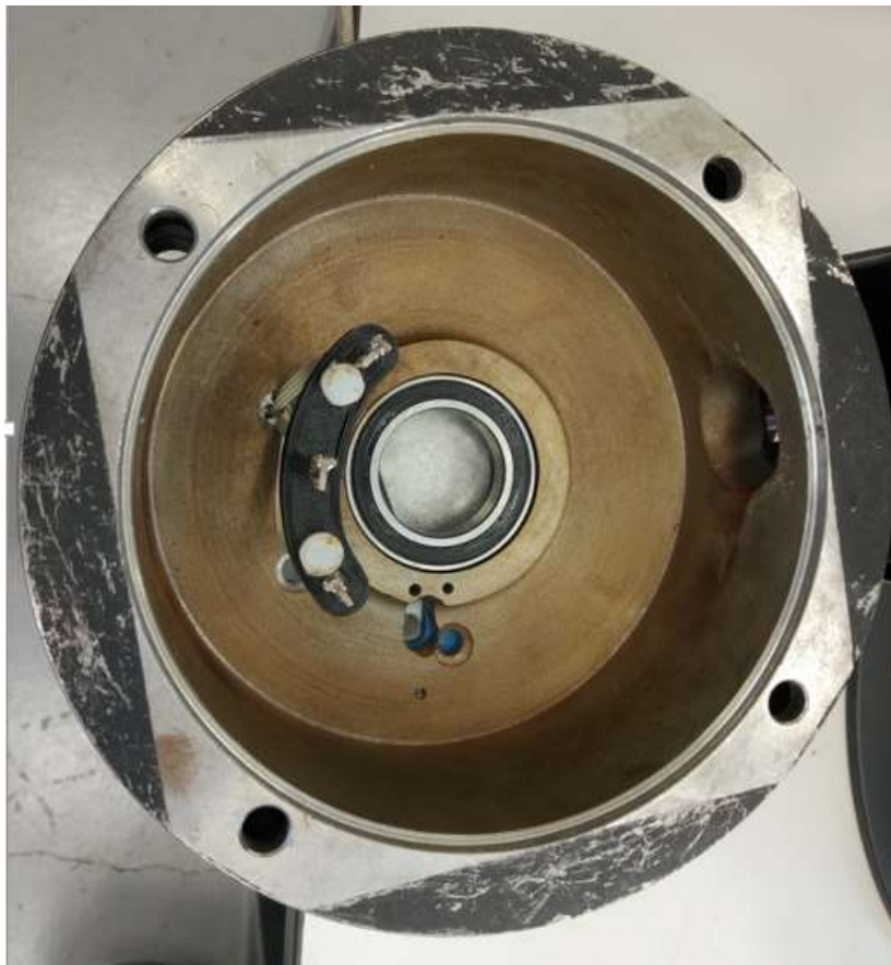
Figure 4.4 - View on the Hall-effect sensors placed on the end shield of the IPM machine.
