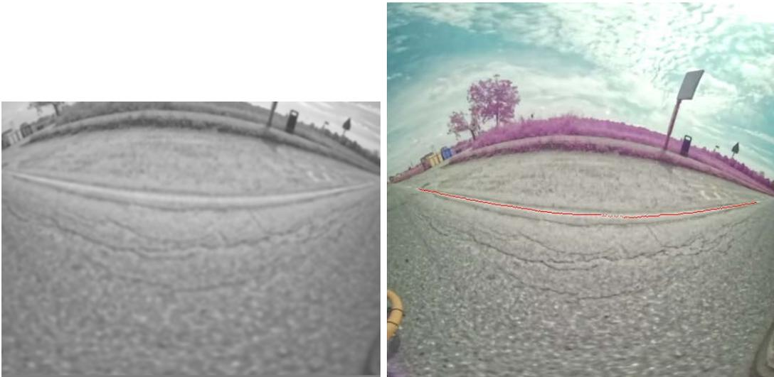
**Figure 6.3:** Faded line not found with traditional CV and correctly detected with CNN.
