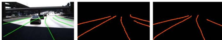
**Figure 2.10:** From left to right: input image, result of ENet-SAD (97.2% of accuracy) and result of SCNN (95.2% of accuracy). Images taken from [35].
