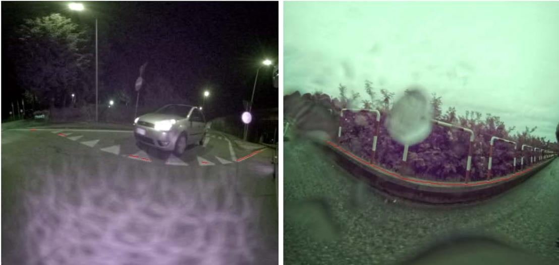
**Figure 5.7:** False positives obtained with the CNN.
