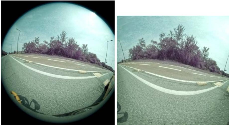
**Figure 3.2:** At left, a captured fisheye image. At right, its representation adopting the spherical model.
