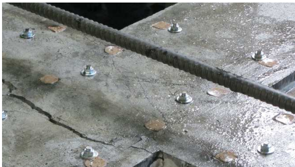
Figure 4.13 – Bending failure in the beam and several micro-cracks in the joint area
