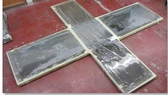
Figure 3.18 - Curing conditions of precast panels
