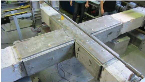
Figure 4.11 – JPC-R after test
