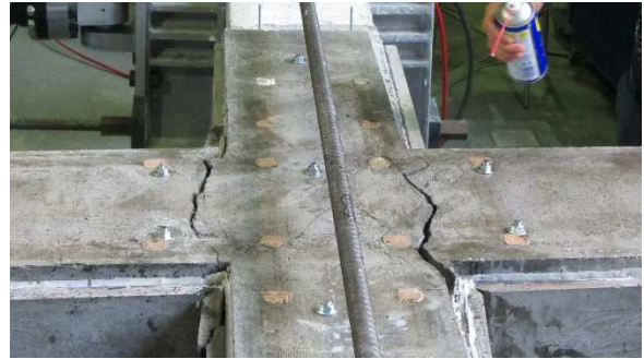
Figure 4.12 – Bending failure in the beam
