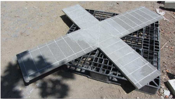
Figure 3.23 – surface not completely roughened
