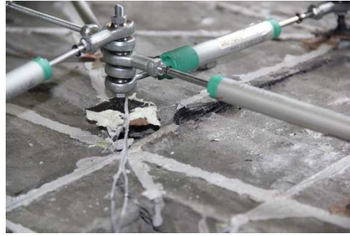
Figure 4.19 – Failure of the longitudinal bars, JPA-3
