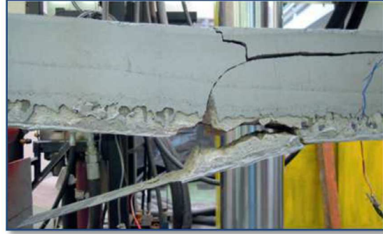
Figure 2.9 - brittle failure mode due to epoxy-concrete debonded [13]
