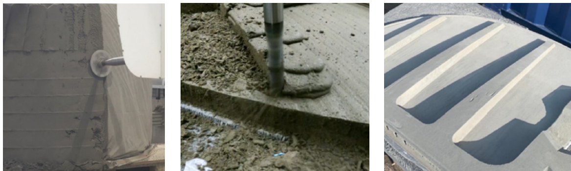
Figura 11. Digital trowelling; Digital milling green-state; Digital milling: risultato finale a materiale indurito (Lowke 2024).
