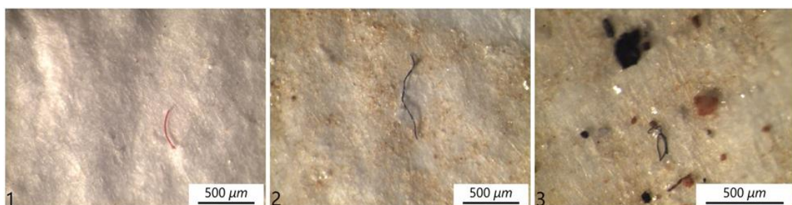
Figure 4.86. Pictures of microplastics found in MOC2. 1.Red fibre; 2. Blue fibre; 3. Black fibre.
