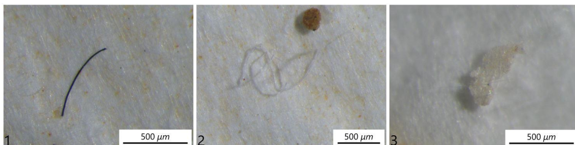
Figure 4.4. Pictures of microplastics found in MOC13. 1. Blue fibre; 2. Transparent fibre; 3. Transparent film.
