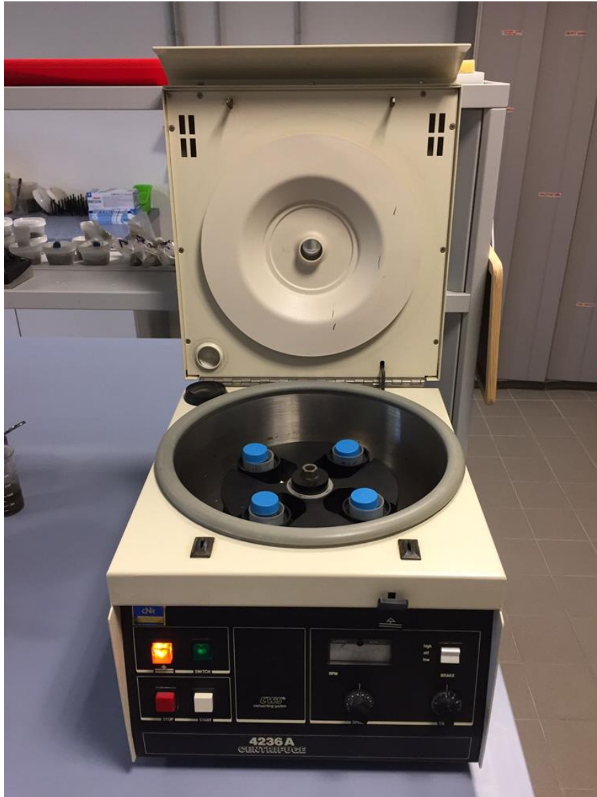
Figure 3.4. Centrifuge machine used to enhance the separation process.
