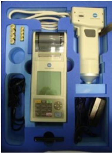
*Figura 33 Colorimetro Konika Minolta*
