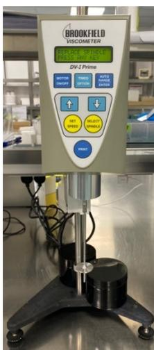
*Figura 32 Viscosimetro Brookfield*
