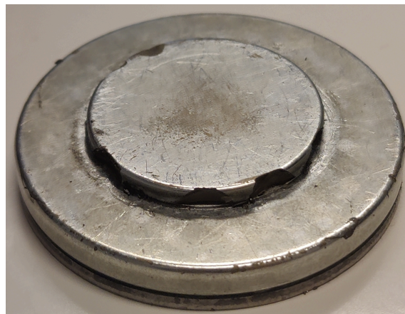
Figure 8.1: Damages on the levitating magnet
