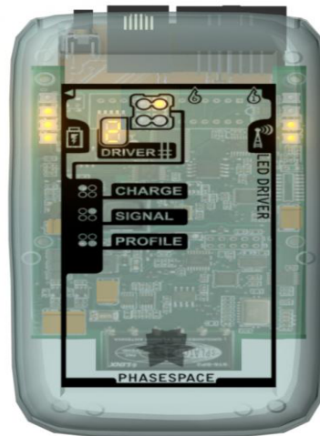
Figure 3.3: LED Driver Unit: it allows to connect up to six LED strings through the 14-pin connector.
