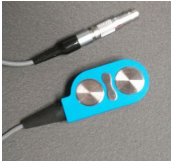
Figure 2.1: Active surface EMG electrode in bipolar configuration from Motion Lab System, model MA-411-003.
