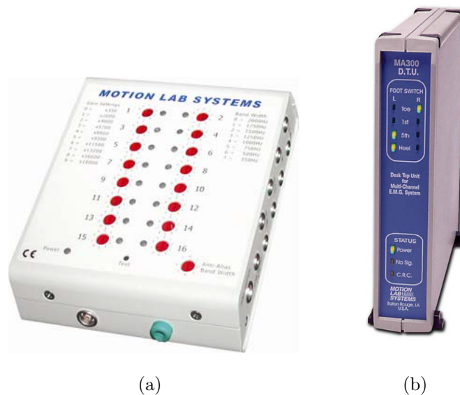
Figure 3.1: The Motion Lab System MA300-XVI: the backpack (a) and the desk-top interface unit (b).
