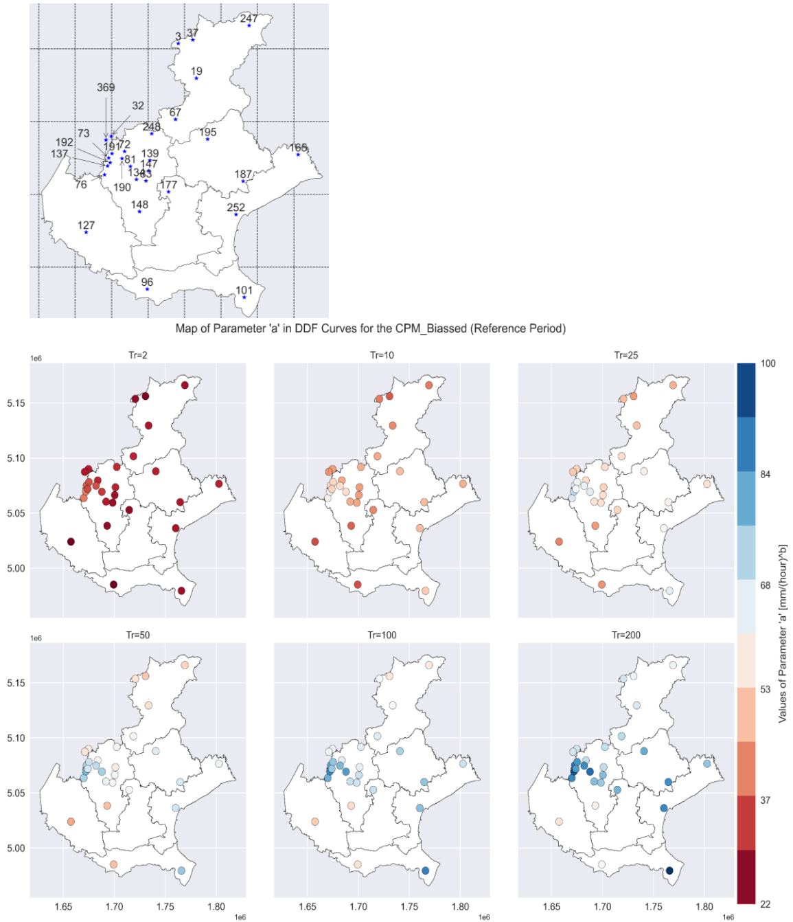
Figure 3-32: Map of coefficient 'a' of DDF curves for biased CPM historical (1996-2005) for various return periods.
