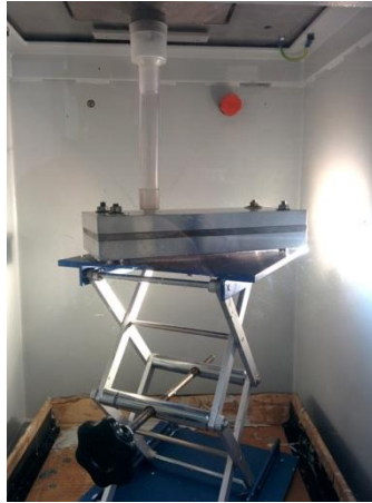
Figure 2.10: mould of 120x50x6[mm] sample during the operation of vacuum casting, lower chamber.
