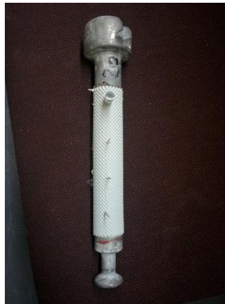
Figure 6.7: good realization of the cylinder textured insulator
