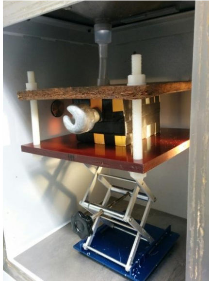
Figure 6.6: fixing of the silicone mould
