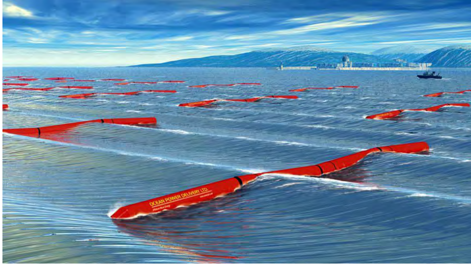
Figure 2- Attenuator device: Pelamis wave farm [7]
