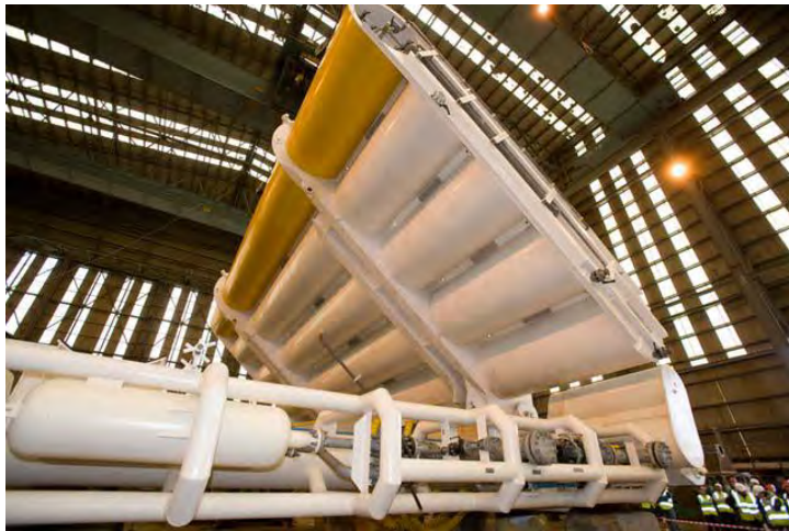
Figure 9- The Oscillator of the Aquamarine Power Oyster [1]
