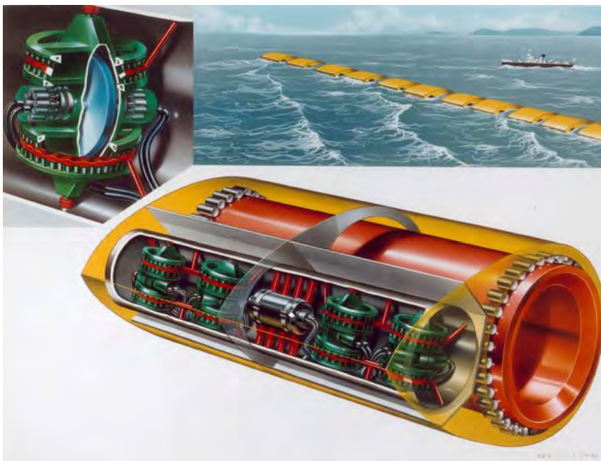
Figure 6- The Duck version of 1979 equipped with gyroscopes (courtesy of University of Edinburgh) [5]
