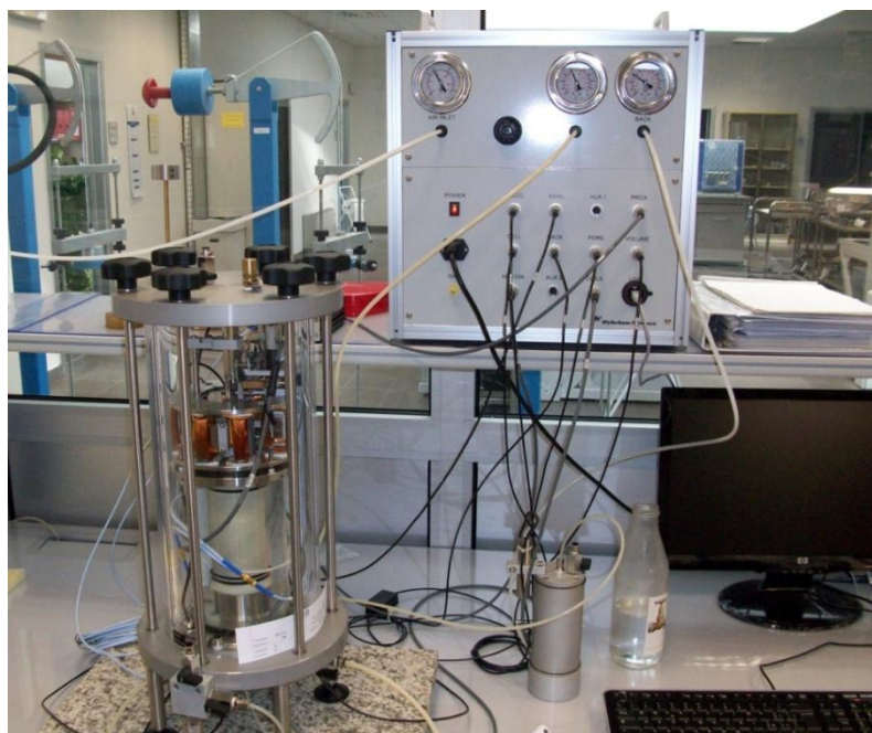
Figure 3.8. Resonant column and cyclic torsional shear devices. To the left there is the triaxial cell. In the middle, at the top, the control unit. In the middle, at the bottom, the device for measuring the volume changes of the specimen.
