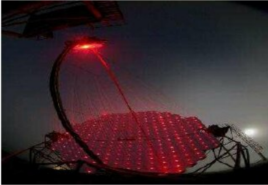
Figure 2.2: AMC lasers activated on MAGIC I, photo taken from (Biland et al., 2007)
