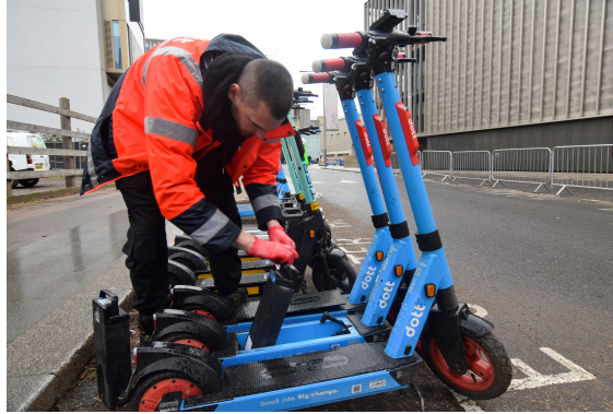
Figure 2.2: E-Scooter easy battery change [8]
