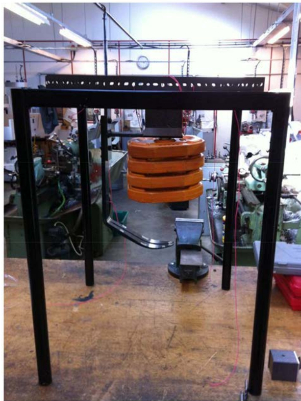
Figure 2.1.5.1 | Prosthesis drop test rig. Dyer, Sewell and Noroozi. 2013 [24]
