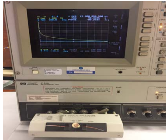
Figure 4.36: Impedance measurement of the capacitive trimmer
