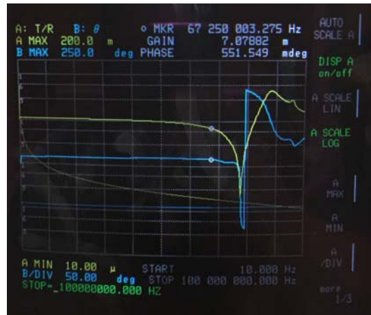
Figure 4.40: Prototype2: cables as short as possible; trimmer partially inserted; about half the full capacity.
