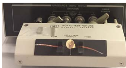
Figure 4.26: Input of the impedancemeter.
