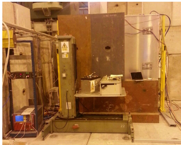
(c) Muon Chamber behind the iron absorber.
