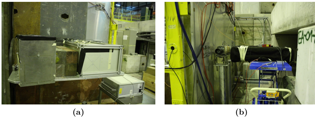
Figure 3.9: (a) A picture of DEVA and \text{PbWO}_4 calorimeters, positioned in front of the iron absorber. Between them, other iron blocks have been added. (b) A picture of the Pb Glass and Cherenkov calorimeters, placed behind the Muon Chamber.
