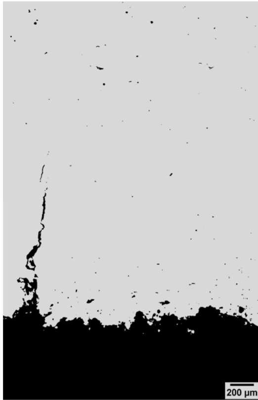
Figure 3.5 Crack that start from the bottom.
