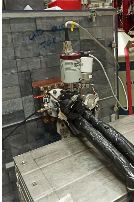
Figure 25: Picture of the target chamber's rear side, where the calorimeter is inserted. The black tubes are connected to the refrigerating system that keeps the cold calorimeter side at the desired temperature.
