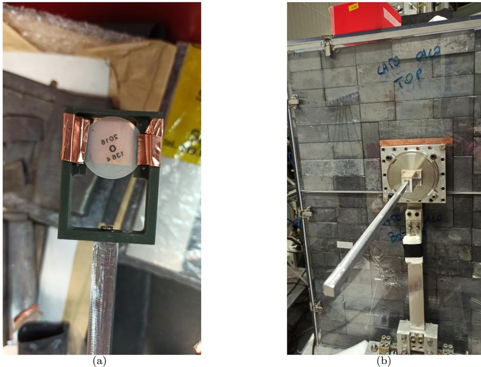
Figure 35: (a)  $^{60}\text{Co}$  source mounted on its holder, which is fixed on a graduated movable flange (b), through which the chamber is closed on the calorimeter side during efficiency measurements.
