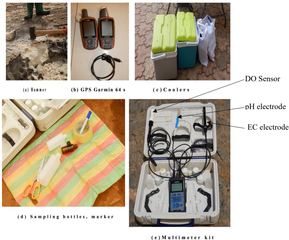
Figure 2: Some equipment used during sampling of the targeted water points
