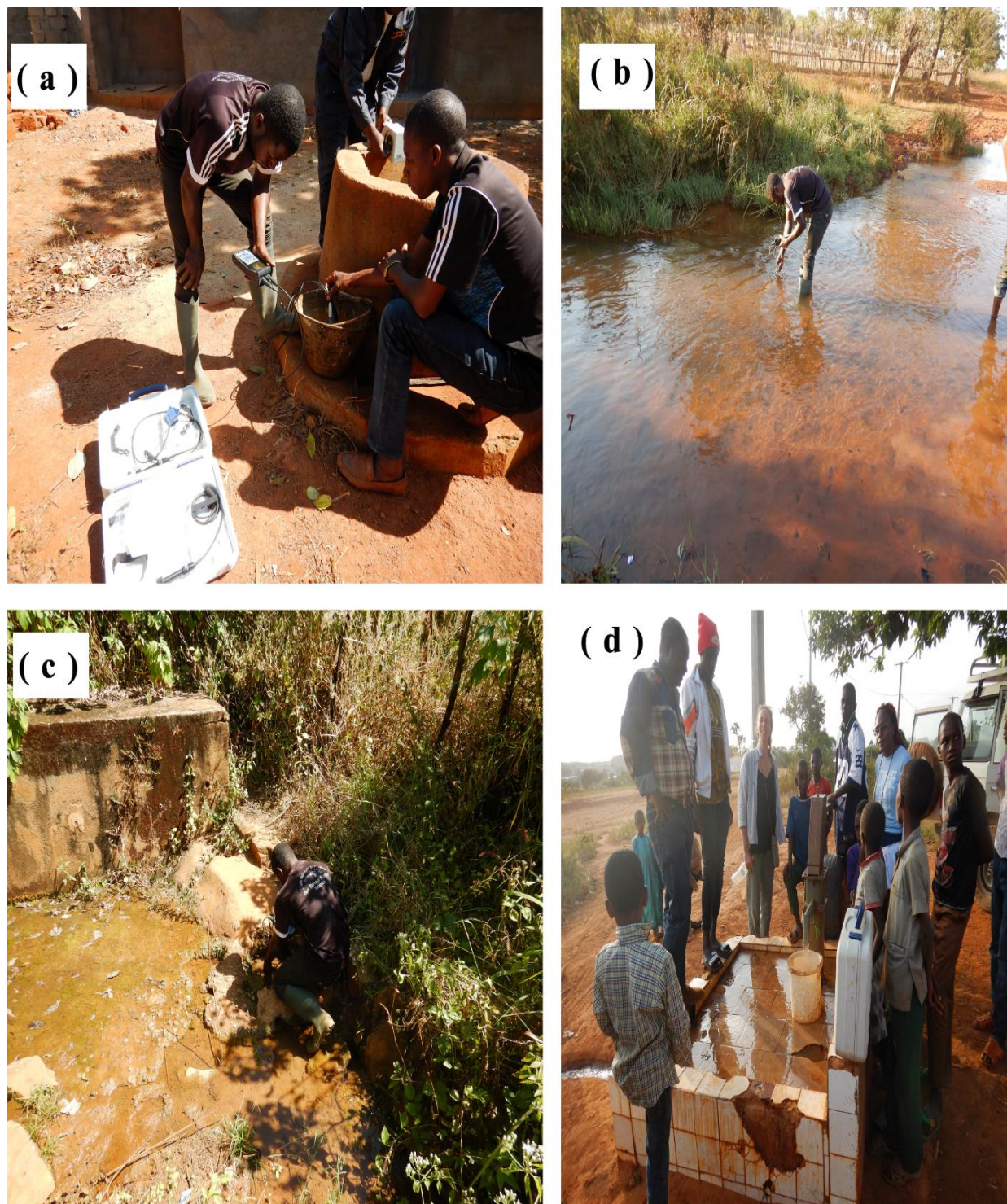
Figure 3: Images showing how some in-situ parameters (pH, temperature, electrical conductivity and redox potential) were obtained from the different water sampling sources; wells (a), rivers (b), springs (c), and boreholes (d).
