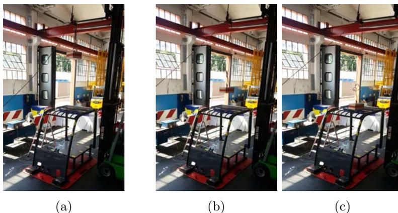
Figura 5.20: Drop Cube Test OHG 3
