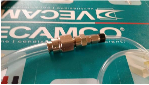
Figure 11: The metallic connector used to connect pipes during the final experiment.
