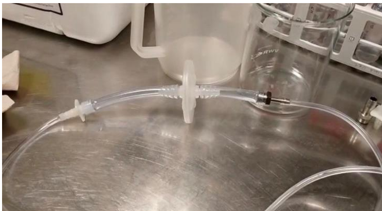
Figure 10: Air filter connected to the small pipes. This picture was taken during the set up, when the use of plastic and metallic connectors were both considered.
