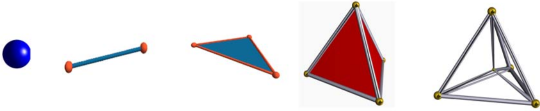
Figure 4.4.: Some simplices: point (0-simplex), segment (1-simplex), triangle (2-simplex), tetrahedron (3-simplex) and 5-cell (4-simplex).
