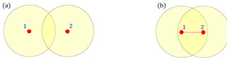
Figure 7.1.: (a) Robots can't see each other, and hence have no way of detecting that their disks of visibility overlap. (b) Robots can see each other, and hence know that their disks of visibility overlap. Visibility is represented by the dotted magenta line.
