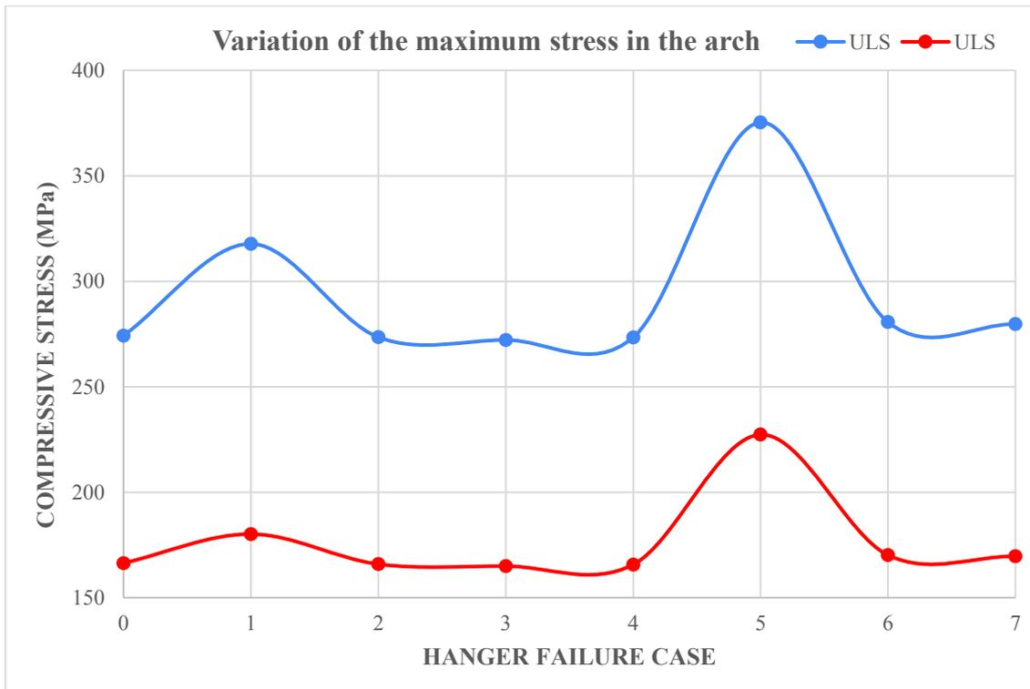
Figure 3.25. Variation of the maximum stress in the arch for the different cases
