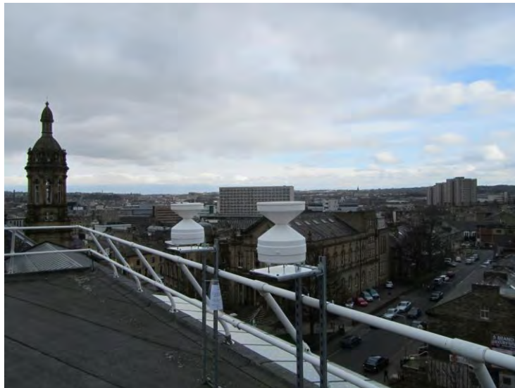
Figure 3.2 Tipping-bucket rain gauge of the University of Bradford located in the point C (see figure 2.1)
