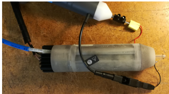
Figure 2.3: The probe connected to the PCC. The red cable is internally welded to the base of the graphite electrode; the black one, instead, is welded to the ground ring.
