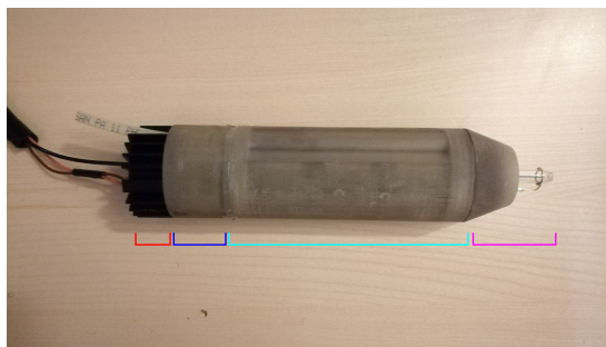
(b) The external body. The main sections can be spot: heatsink (red), circuit (blue), transformer (cyan), nozzle (magenta)
