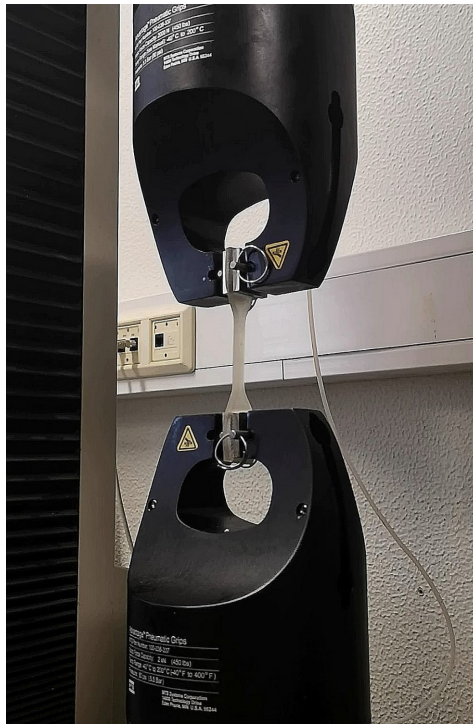
Figure 2.19: Tensile test on a dogbone specimen.
