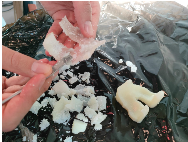
Figure 2.17: Support material removal process.
