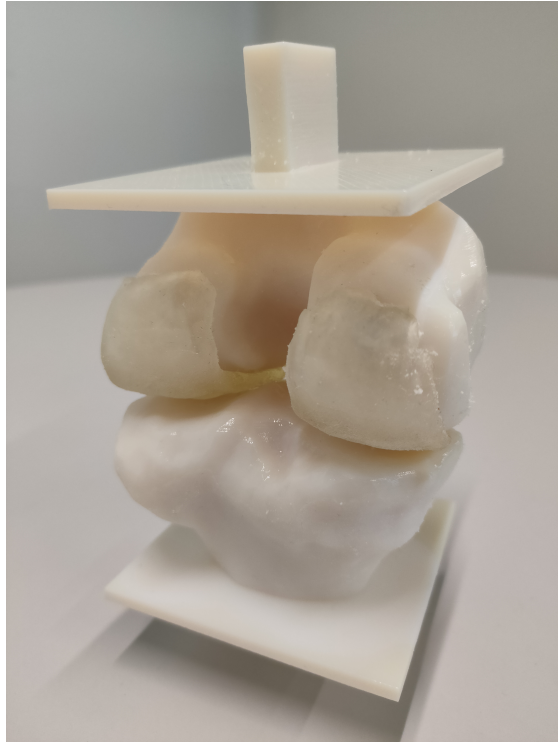
Figure 2.18: Printed anatomical supports and femoral cartilage from subject 18 (Degenerative).
