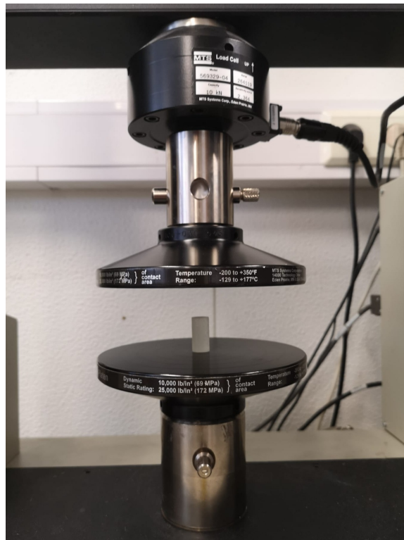
Figure 2.20: Compression specimen right before testing.
