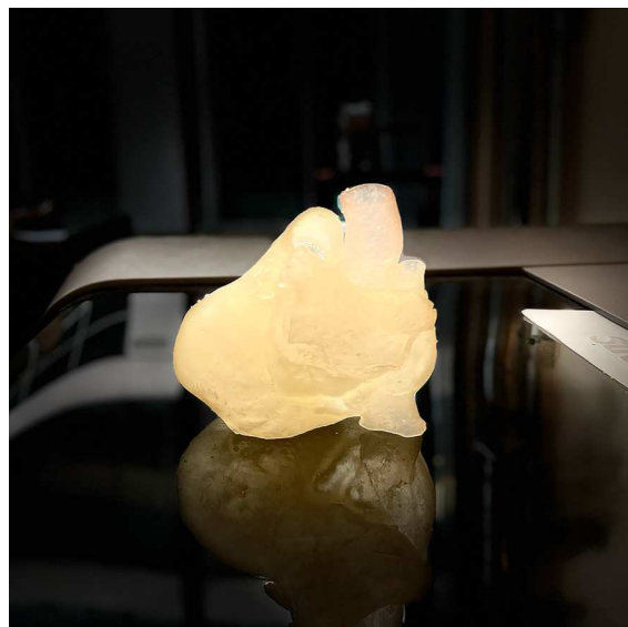
Figure 1.12: Example of a heart printed with Stratasys j850 DAP at Reykjavik University.
