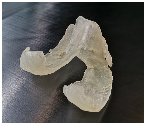
Figure 2.7: Detailed view of a degenerative cartilage printed with the J850.
