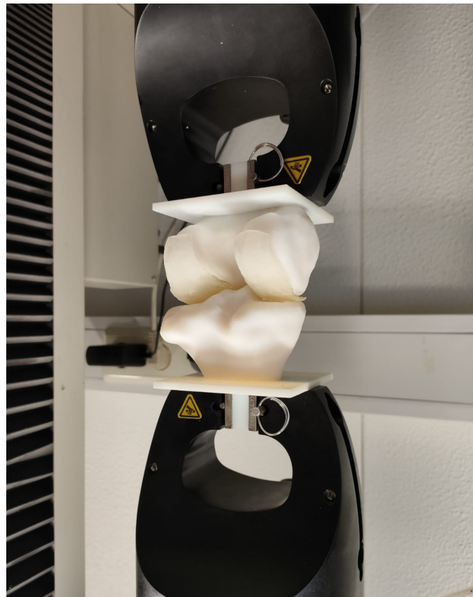
Figure 2.21: Anatomy specific testing setup.
